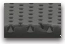
100 Million nano-cones field on a silicon chip emitting digitally controlled electron streams under low voltage
